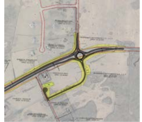
Figure 12 Concept design for proposed roundabout at Montresor Road with connecting to Limestone School Road
